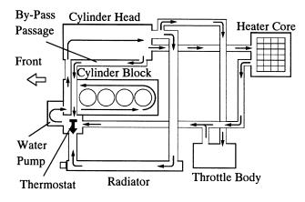
Figure 15. Cooling System
