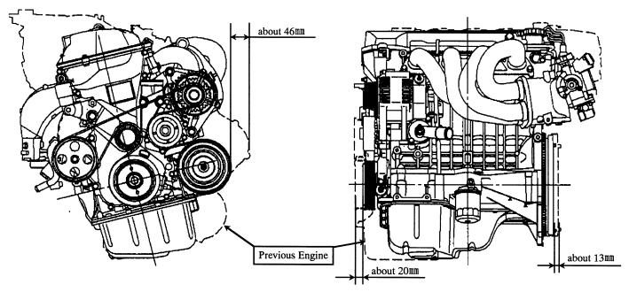
Figure 5. 1ZZ-FE Appearance and Comparison of Dimension
