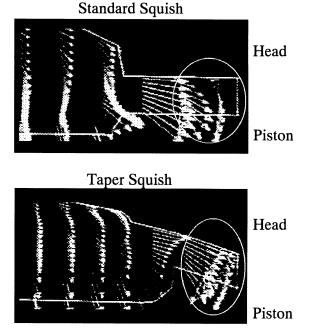
Figure 13. Comparison of Flow Velocity at Squish Area (CFD Simulation)
