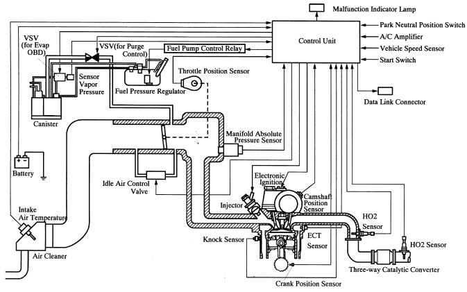
Figure 21. Engine and Emission Control System
