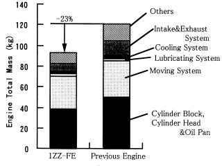
Figure 17. Engine Mass Comparison
