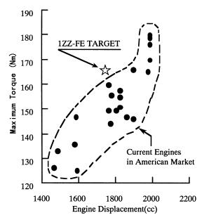
Figure 2. Maximum Torque Comparison
