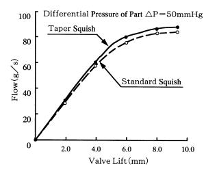
Figure 11. Comparison of Flow Rate Characteristics
