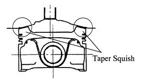
Figure 10. Taper Squish Combustion Chamber
