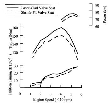
Figure 9. Effect of Laser-Clad Valve Seat
