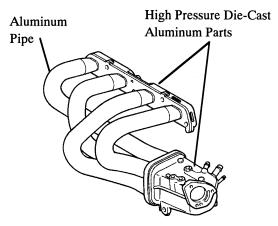
Figure 16. Intake Manifold
