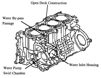
Figure 18. Cylinder Block
