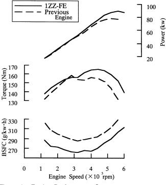
Figure 6. Engine Performance Curves
