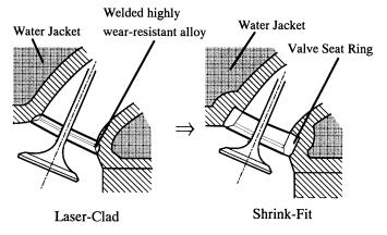
Figure 8. Adoption of Laser-Clad Valve Seat
