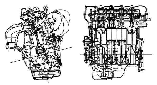
Figure 4. 1ZZ-FE Engine Cross-Sections
